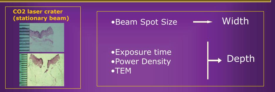
**TEM 00:** The irradiance across the beam is distributed in a **gaussian fashion** peaking at the center of the beam and falling off to zero at the edges.
